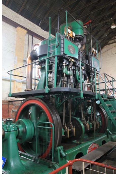
Psyche Bend pumping engine 1891 at Mildura supplied water for irrigation. Recommissioned 1995 for display purposes.
